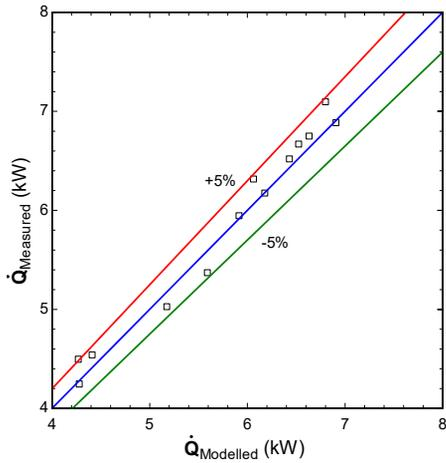
**Fig. 3: Experimental vs. theoretical heat transfer rate**
